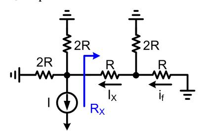
• With similar analysis, it can be shown that the current through  $b_4 \& R_f$  is I/8. Therefore,
